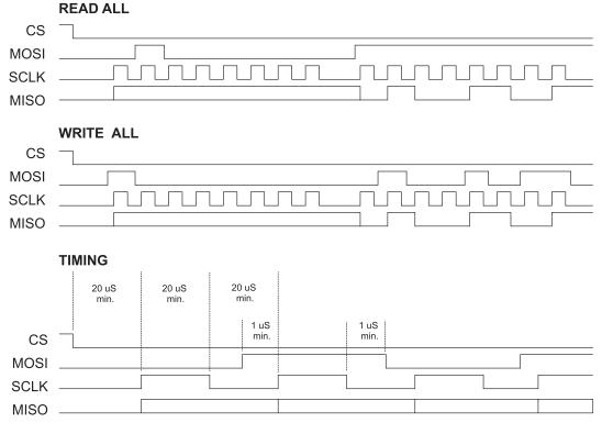
Figure 2.7.1: SPI Timing
